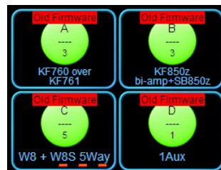
Figure 26-7: Old Firmware Notification in the Lake Controller
