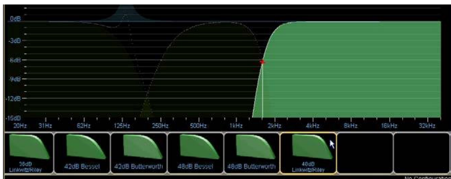
Figure 4-49: Changing the crossover slope
