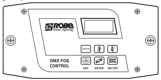
**DMX Fog Control:** 10 meter wired multi-function remote control module with 5-pin XLR connector for ROBE Fog 1500 FT. Its interface allows the operator to customize fog machine functions by adjusting fogging duration, interval and volume. Its LCD displays current operating parameters, which are automatically stored in non-volatile memory, allowing the machine to be powered down without losing function settings. Instructions below:
